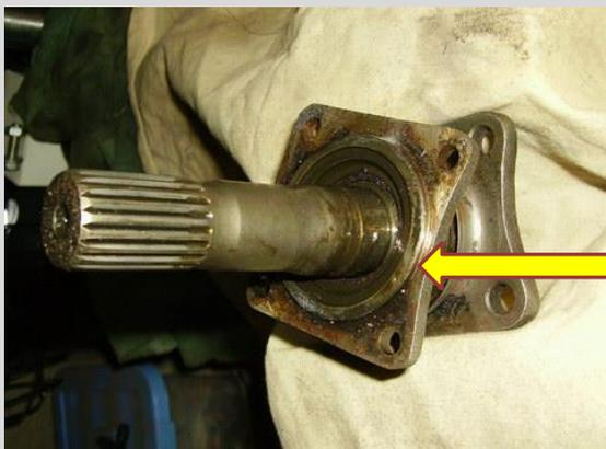
Retirer la plaque du support du joint spi.
