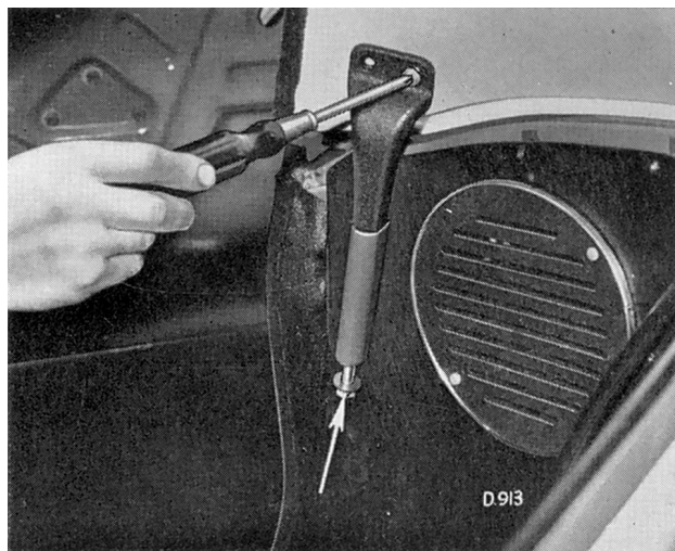
Fig. 54. Side bracket attachment (Spitfire 4 and Mk. 2)
